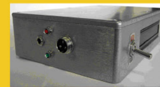
CARINA (Ohmmeter for train coupled axle electric resistance measurement)
