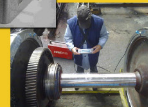
CARINA (Ohmmeter for train coupled axle electric resistance measurement)
